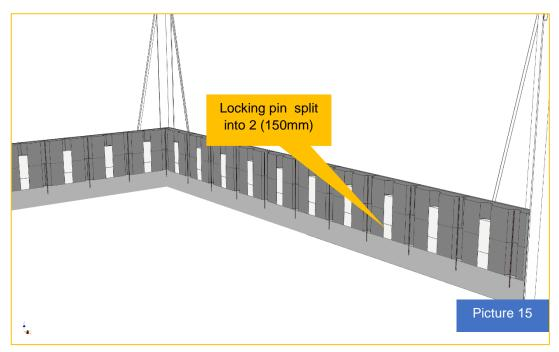
"Picture 15" shows cross sections of the rear wall. We start by dividing the entire locking pins in half. The locking pin should be inserted into all holes where no rebar is inserted. No more locking pins should be inserted in this level at this time (only 1/2 pin in the first shift). Holes under the door in this description can be filled with a whole locking pin.
