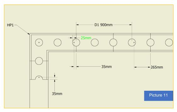
Technical drawing shows that in the case of "Figure 10" the rebar that is placed on each side of the door should have sufficient concrete covering. Marked in green shows 25mm from the centre of  $\emptyset$ 12mm rebar and against the wall in the hole. The distance can then be measured to 25mm minus 6mm = 19mm cover. Minimum reinforcement cover should not be less than 15mm. The same principle also applies to windows and gate in this example. How we proceed we get back to.
