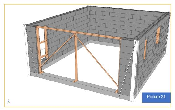
Principle \* / proposal for bracing the gate. (\* more bracing is required in the door opening) Should the work stop along the way or in the event of heavy rainfall, the block should be covered on top with a strip of plastic / cardboard to avoid collecting water.
