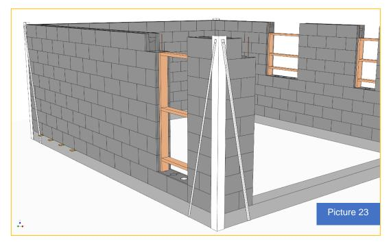
Stiffening of door, window and door openings is done easily with 146x48mm supports, the bottom beam should be set up so far that you can fill concrete in the column below, this is especially important in window openings. The reason why columns under doors and windows are cast out is that the blocks should work homogeneously together. Some window manufacturers also require torque points for large windows / doors. Then place the rest of the U-BLOC over the door and windows.
