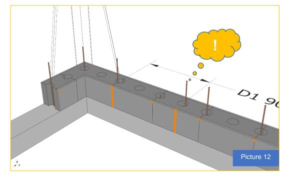
"Figure 12" Indicates that concrete pillars do not go up every 60cm then it should be exchanged with 2 concrete pillars every 30cm. Never use 2 pillars with eps locking pins consecutively without consulting the designer engineer.
