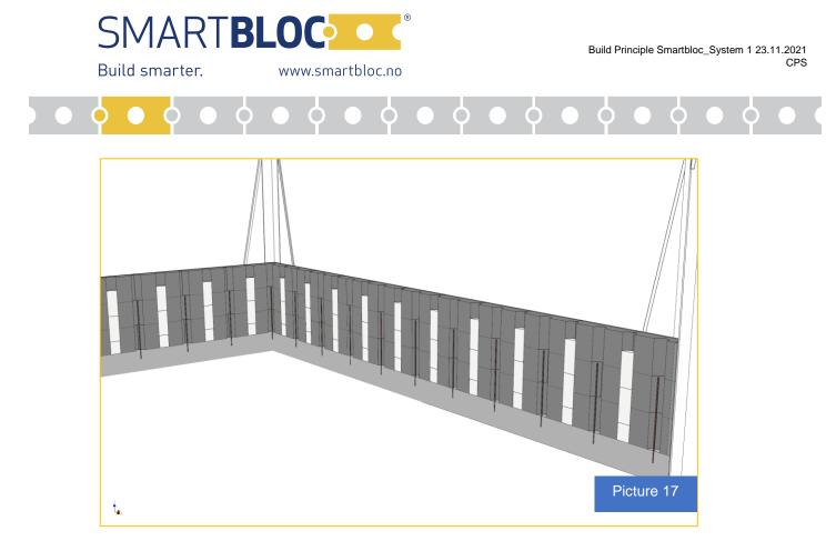
"Picture 17" shows cross sections of behind the wall after 3 levels of blocks. After level 1 is set and 1/2 locking pin is set we place blocks in level 2. Full-length locking pins are mounted after the blocks are set. Next, we repeat the procedure with level 3 before we put the locking pins (full length). The same procedures apply the next levels. The reason we put locking pins after the blocks have been placed is to avoid that the locking pins push the blocks apart before they are placed.
