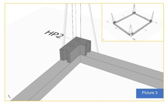
L-BLOC is put in every corner. Check that the direction of the L-BLOC is correct so that the measurement between the L-BLOC (corner block) and the next L-BLOC corresponds to the number of N-BLOC (normal block) (the distance can be divided by 60cm and you get an integer) remove locking pins from the L-BLOC. (pre-posted, see figure 8)
