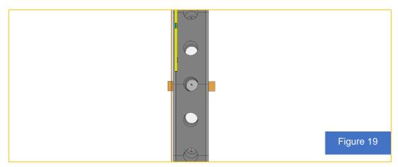
"Figure 19" shows an example of adjustment, with a search of 0.5cm horizontally, this is directed with wedges set against each other, deviations larger than 0.5cm should be arranged before blocking. Wedges should always be placed in the block joint.
