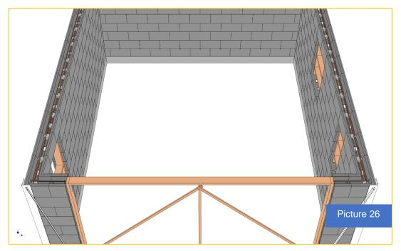
Start in a corner and fill up to <u>4th level</u> and continue around, then fill up to <u>8th level</u>, finally filling the remaining into columns and U-BLOC. To avoid air in the concrete pillars, knock directly on the reinforcement, vibrator can be used on the reinforcement, but <u>do not</u> use vibrator down in the pillars. The filling is done in one operation. PS place the concrete hose in U block and let the concrete flow down into the columns.
