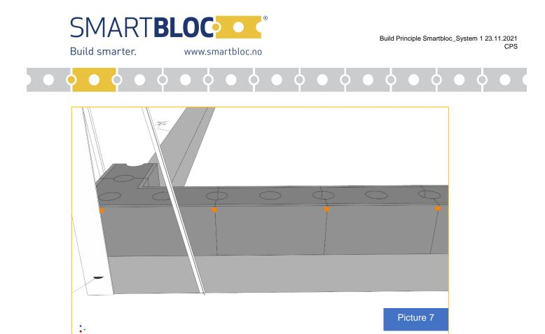
TIP: After doors and windows are marked. So, it is also good practice to mark all holes for concrete pillars. Mark again on the 6th row.
