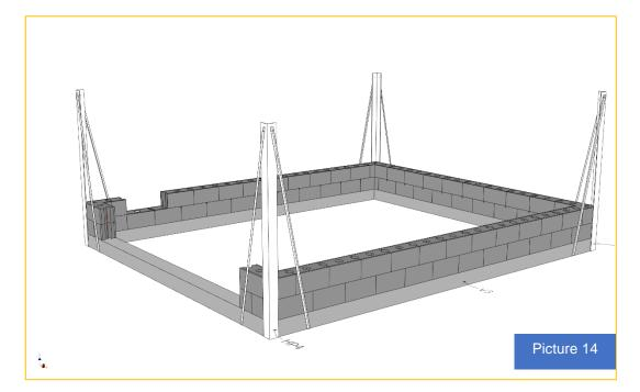
Fill with N-BLOC between all corners. At the door and gate, an N-BLOC is divided into two parts, each of 30cm.
