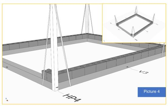
Remove guide pins from the N-BLOC, fill the N-BLOC between corner blocks. (L-BLOC) be sure to push the blocks firmly close together. Keep the direction with masonry cords.
