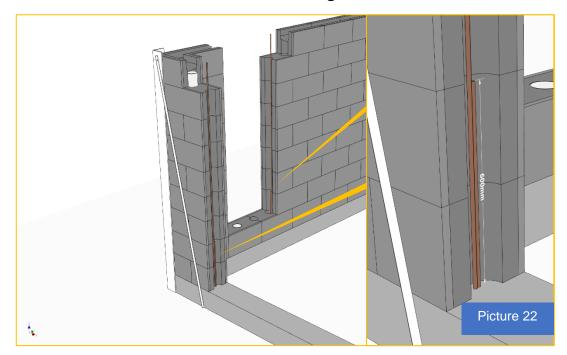
Before bracing, it is recommended to put standing reinforcement in the door, window and gate. To keep the reinforcement in position, use strings that are twisted around the reinforcement and fastened in the block, the top of the reinforcement binned together with reinforcement in the U-BLOC.
