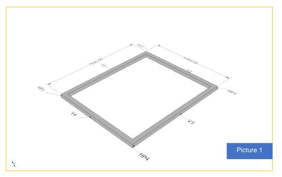
Foundation ready for blocking. Check the diagonal, in this description it is 9795mm
