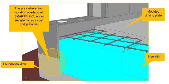
For uninsulated flooring, the floor can be cast against foundation or the first level with SMARTBLOC.
