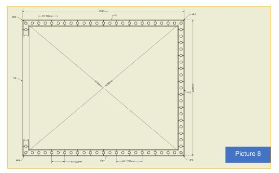
Before proceeding drilling, diagonals are checked. From HP1 to HP3, 9795mm is measured outside edge. The diagonal from HP2 to HP4 should be the same as from HP1 to HP3!
