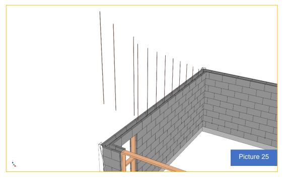
1 or 3 x Ø12mm (with or without backfilling, check table) reinforcement is lowered centrally into empty columns, tied together with reinforcement in U-BLOC, which in this project is 3 x Ø12mm. (2 at the bottom and 1 at the top) NB! Do not drop reinforcement from the top, reinforcement can "bounce" back up!
