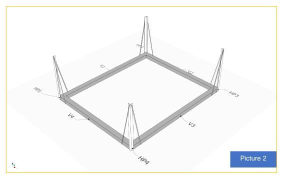
Set corners posts in every corner. In this description, posts made of aluminum profiles are used, but these can also be built with formwork materials.
