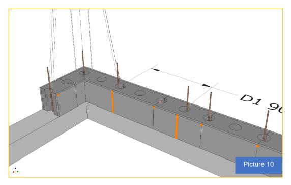
In this description we use an M9 x M21 door (89cm wide x 209cm high) the opening is 90cm. For the best possible fixing for door frame, cast half concrete pillars on each side of the door.
