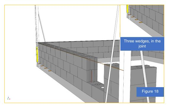
"Figure 18" shows the example for adjusting the wall between HP1 and HP2 tilt out approx. 0.5cm, this is aligned with wooden wedges. Wooden wedges used should be 5-10cm wide. wedges should always be placed in the block joint, not in the middle of the block.
