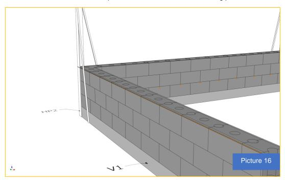
Block like this up to 3 more levels, the use of masonry cords makes it easy to keep the direction.
