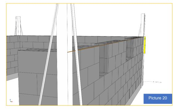
Block then upwards. Keep an eye on the masonry cord and horizontal level, remember to put whole guide pins after each shift with blocks.
