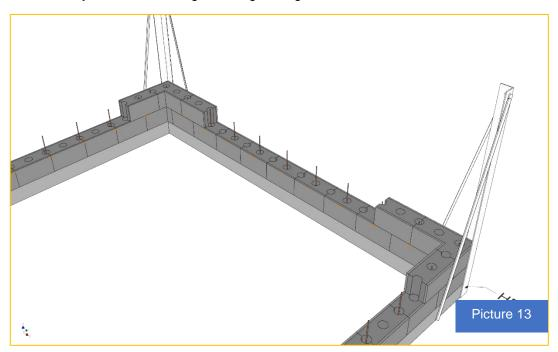
Reinforcement is placed out into the remaining holes. Then build up other levels with blocks, starting in each corner.
